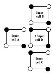
Figure 5. the input cells and output cells of a majority voting gate.
