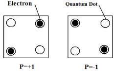
Figure 1. standard QCA cells showing the polarizations of two ground states.
