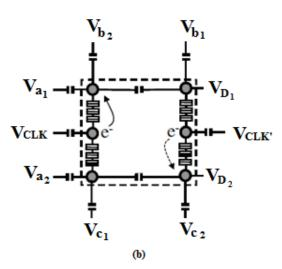
Figure 4.(a) A Realization of a basic QCA cell composed of quantum dots, tunnel junctions and capacitances. (b) Shematic diagram of a clocked three-input majority gate circuit.
