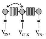
Figure 2. When the clock signal is on, electron tunnels to the dot with positive potential
