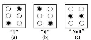
Figure 3. A clocked QCA cell that is a six-dot cell.(b) varying the potential of the middle dots or pulling the electrons onto the middle dots leads to a "null" state of the cell, (a) ,(c) and by varying the potential of the middle dots or by pushing the electrons off of the middle dots state of the cell become"1" or "0".
